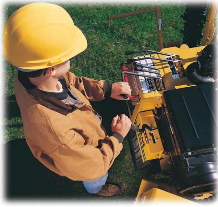
**Insulated, color-coded controls** help protect the operator against shock injury from electrical strikes. The separate, color-coded controls for steering and propulsion provide operators with a quick, visual reference.
